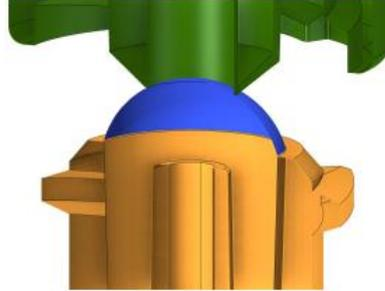
Figure 1. Illustration of a meniscus (blue) on the surface of the LDT syringe hub (yellow)
