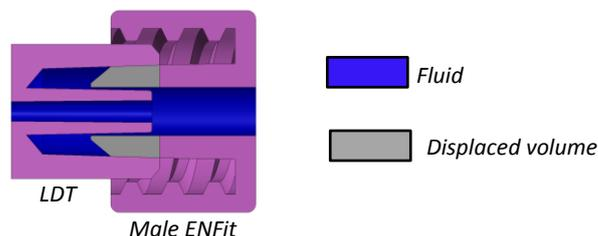
These volumes will be quantified in min / max tolerances via the SOLIDWORKS® CAD modeling.
